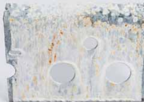
Significant white rusting across entire part as well as many spots of surface red rusting
