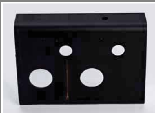
Minimal rust at scribe
