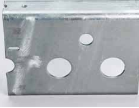
Treatment over a cleaned cross-member
