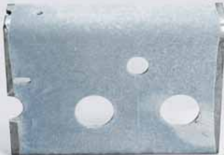
Significant white rusting - no red rusting
