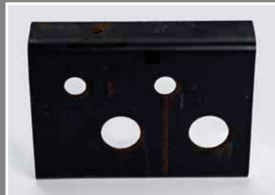
Significant rusting and blistering
