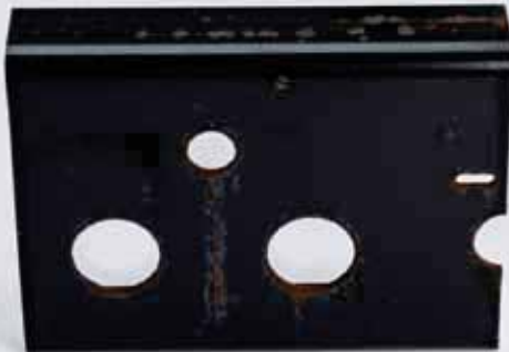
Significant rusting and blistering
