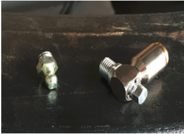
Fig.: 3 - Prepare new fittings
