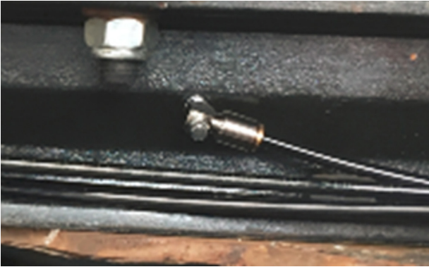
Fig.: 8 - Cut grease hose to required length
