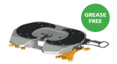
The "No Lube" technology means that this ductile cast iron fifth wheel with NoLube wear plates does not require regular greasing, the same is tru for the special NoLube components in the locking mechanism and the bearing inserts between the fifth wheel and the mounting brackets.
