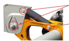
The surfaces of the hanger bracket that contact the pivot bolt washers and upper shock absorber bolts and nuts must not be painted.
