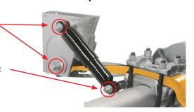
This restriction is an industry standard that is not specific to SAF-HOLLAND suspension components. The reason is that any paint applied to the surfaces of bolted connections can compress over time, potentially causing a loss of torque at the bolted connection, which may lead to damage to components. Accordingly, failure to comply with this restriction may affect SAF-HOLLAND warranty.
