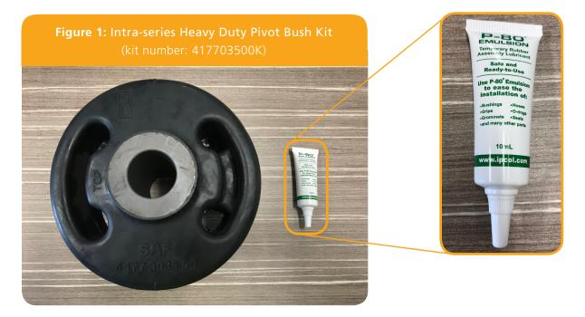
The assembly lubricant is used to facilitate installation of the bush into the trailing arm. The contents of the tube should be applied to both the outside of the bush and the inside of the trailing arm immediately prior to installation.
