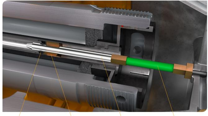
Double-lipped radial seal prevents air system leaks into the wheel end. Heavy-duty bronze bushing assures proper alignment of rotating shaft. Polished steel rotating shaft provides a smooth, long lasting sealing surface. Flexible PTFE tubing withstands extreme temperatures.
