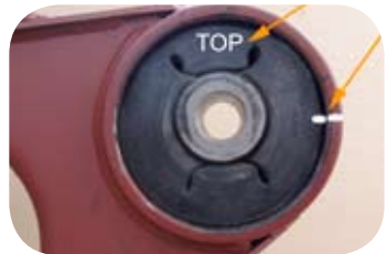
Fig. 14 · Checking the installation position
