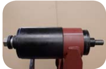
Fig. 6 · Removal tool installation
