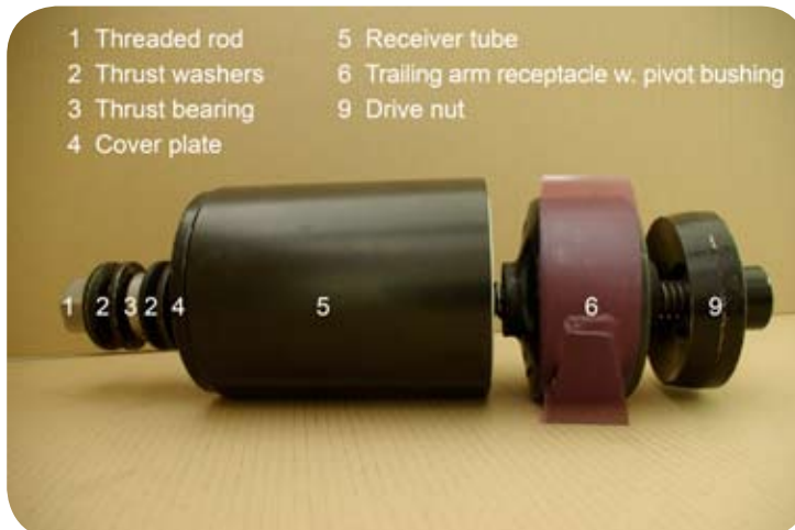
Fig. 1 · Identification of removal tool components
