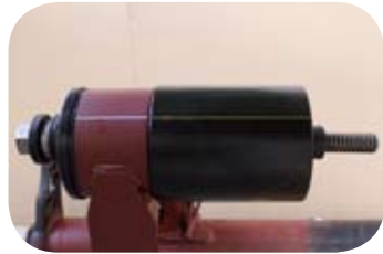
Fig. 15 · Correct receiver tube position
