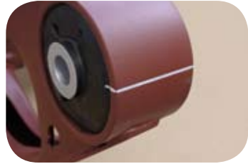
Fig. 5 · Marking the bushing orientation
