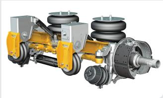
The light, simple and durable design of the SAF heavy-duty PosiLift™ provides a twin bag lift solution where a conventional Center Bag Lift will not fit within the trailer chassis (e.g. hoppers, bottom discharge bulk tankers, etc.). The lift system allows the self steering axle to be lifted while backing up, and for tight maneuvering in a yard, or when running empty (as regulations allow).
