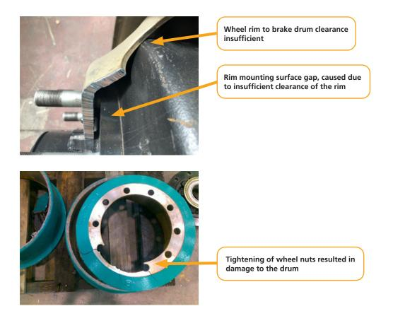
In the past SAF-HOLLAND has had issue reported involving the use of DOT-T and DOT-E standard rims. It is the responsibility of the installer to ensure correct clearances when installing rims.
