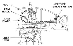
Apply grease to lock jaws and front of throat directly or through lube tube grease fitting.
