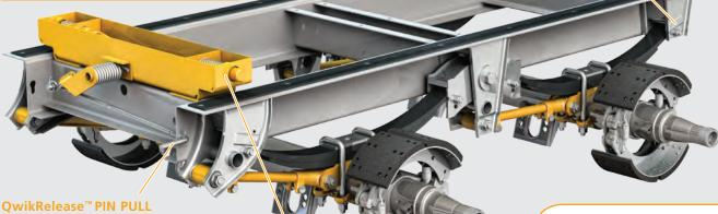
The low pull effort of the release handle makes slider adjustment safe, easy and efficient. Patented design allows for one driver slider repositioning and eliminates the problem of releasing bound-up pins.
