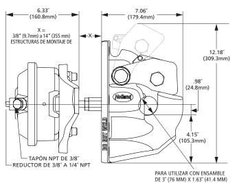
DE DIÁMETRO INTERIOR 6.50" (165.1 mm) 5.0" (127mm) 3.25" 2.5 (82.6mm) (63.5mm) $\oplus$  $\oplus$ 4 25 10.65" (270.6mm) (108mm) .38″ (9.5mm)  $\oplus$ 2.38" (60.3mm)  $\oplus$  $\oplus$ 5.18" (131.5mm) (54mm)  $\oplus$  $\oplus$ .82″ (20.8mm)
