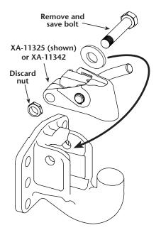
Clean and apply Never-Seez® to entire shaft of pivot bolt (not on threads).
