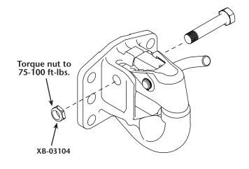
Check latch for proper operation. When closed, latch dog must automatically engage under lip as shown.
