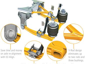
Maintenance free welded axle adapters save time, cost and weight.
