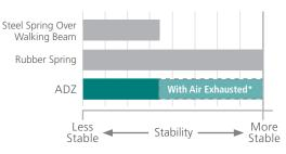
\* When fully loaded vehicle is in stationary position and on uneven terrain, or when dumping, the air can be exhausted from air springs to increase stability of vehicle. Typical air ride will match stability of a rubber spring under air exhausted conditions.
