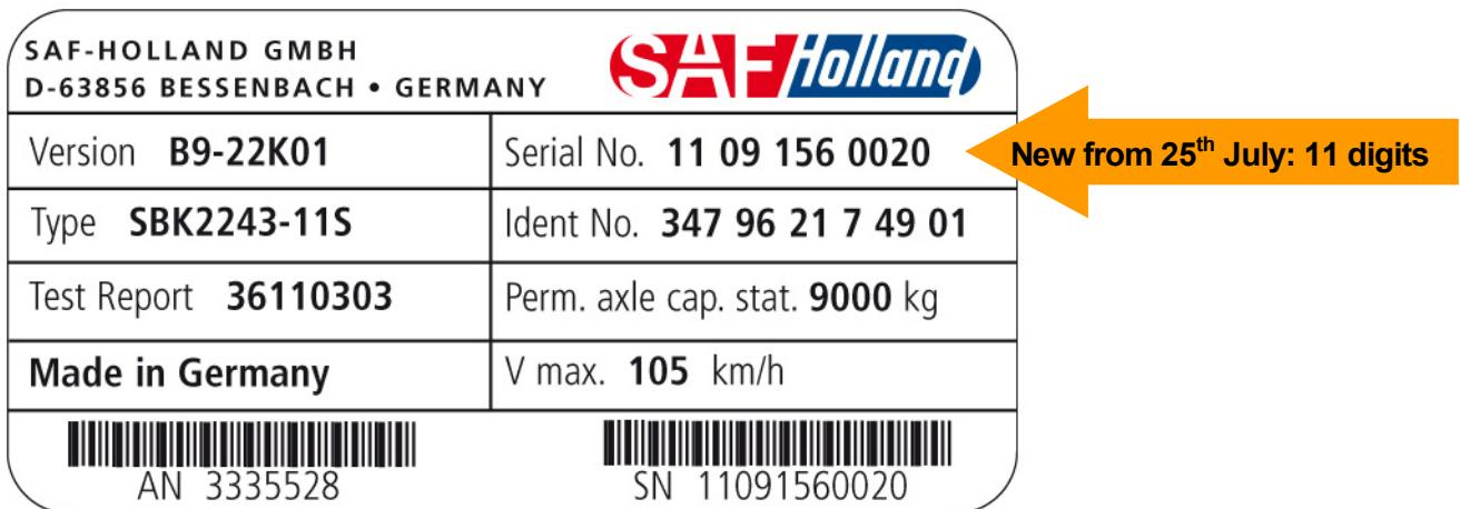
Fig1: SAF-HOLLAND axle type plate from 25.07.2009
