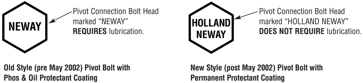
Figure 3. Pivot Bolt Torque Lubrication Requirements - Old Style vs. New Style Identification
